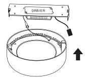
Close the fitting by turning it clockwise, open it by turning it counterclockwise
